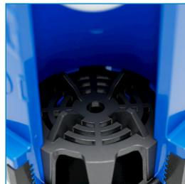
The **air release valve “ECO” double effect** protects your installations, given its ability to release air and admit it under vacuum conditions. Its closing ball allows a perfect closing at low pressures and the prefilter, provides additional protection against water dirt and solids suction when acting against vacuum.
